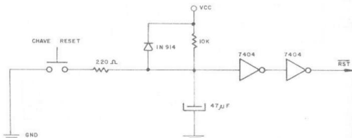
Fig. 8.2 - Chave RESET e Circuito POC.
