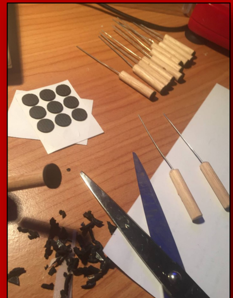
For the 'fret fingers' I cut wooden dowel, drilled a small hole in one end of each and glued a straightened out paper clip into the hole. At the other end I glued rubber feet (that had to be trimmed down a bit with scissors).
