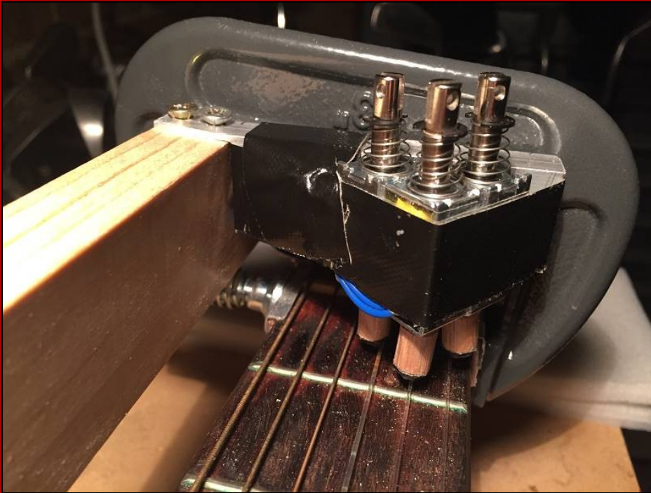
Here is a test I did with 3 solenoids that proved to be unsuccessful. While they moved quickly down to the strings when powered on, the pressure was simply too light and the note when played sounded very muffled. I abandoned this idea and switched to using servo motors instead.
