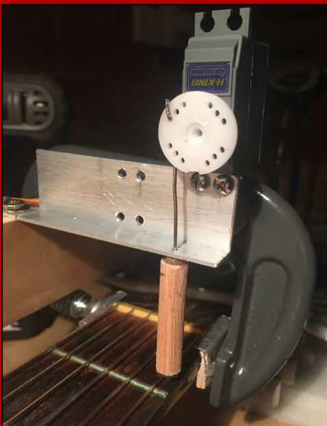
Here is a test of one of my 'fret fingers'. The paper clip has a small bend to feed through the cam on the servo. When the servo turns through about 60 degrees, it either pushes down on the string or lifts away and the sound of the note when played is very good.
