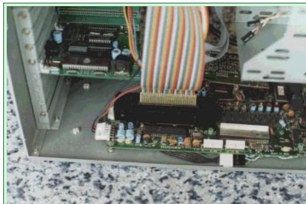
The interface mounted in a MSX which is in a pc desktop case.
