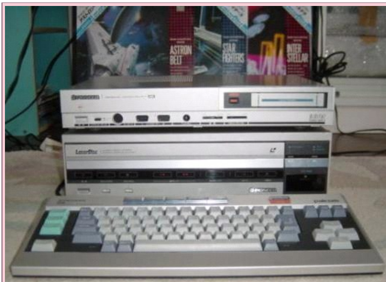
The Pioneer Palcom PX-V7, with the LD-700 Video Disc Player underneath it and some games in the background.
