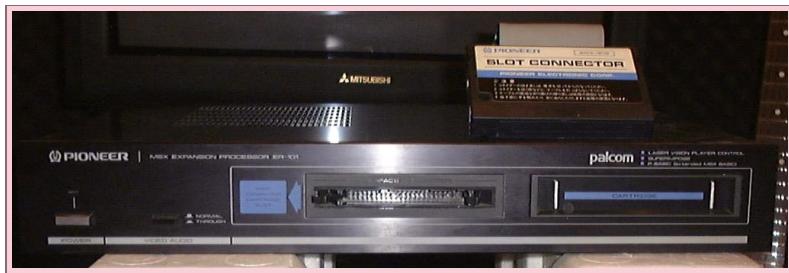
The ER-101 is almost an MSX computer on itself! It sort of makes your MSX a Pioneer PX-7. It includes 'Laser Vision Player Control', 'Superimpose' and 'P-basic (extended MSX-basic)', just like is built in in the PX-7.
