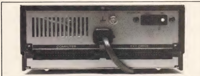
Above: Back of the drive showing the sockets. Right: Microflops. Below: The cartridge interface cable
