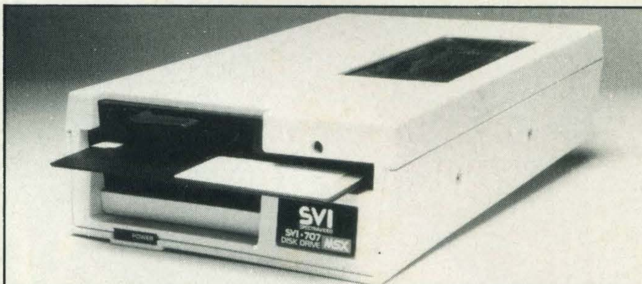
Spectravideo's first drive was a 5.25 inch model. The track and sector configuration can be very different from a 3.5 inch drive
