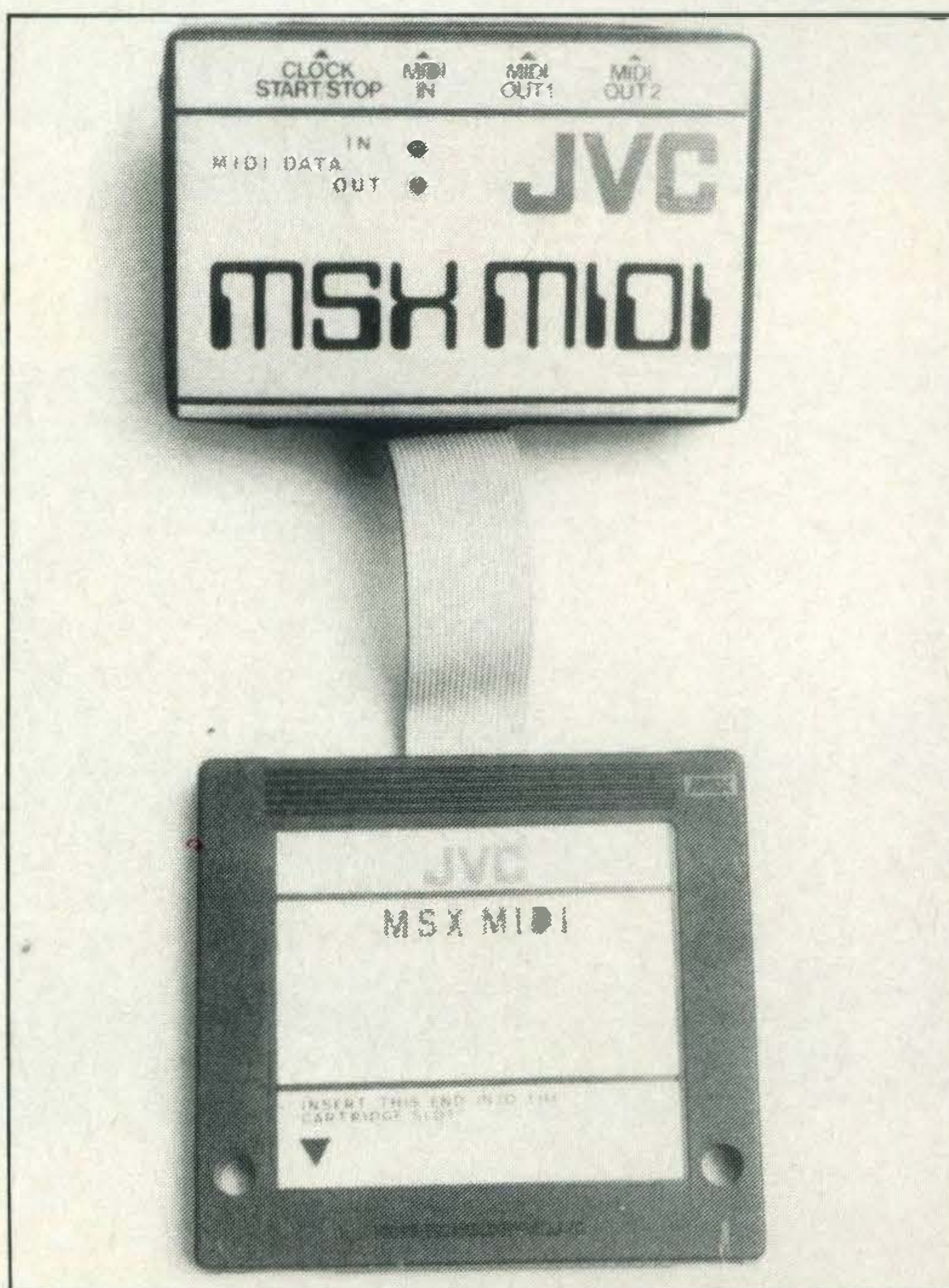
The MIDI interface slots into the cartridge slot
