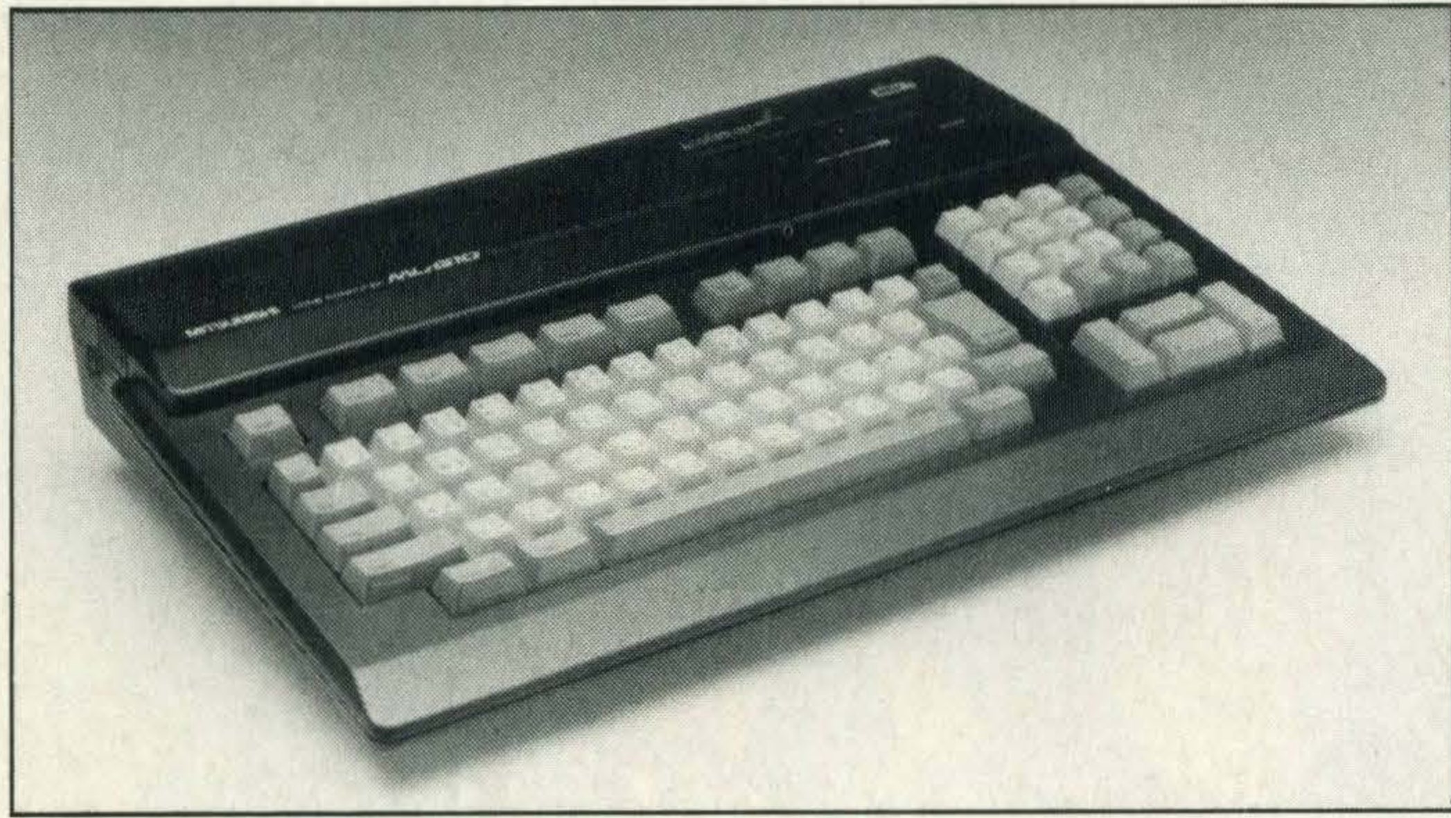
Mitsubishi's prototype MSX2 micro with separate numeric keypad
