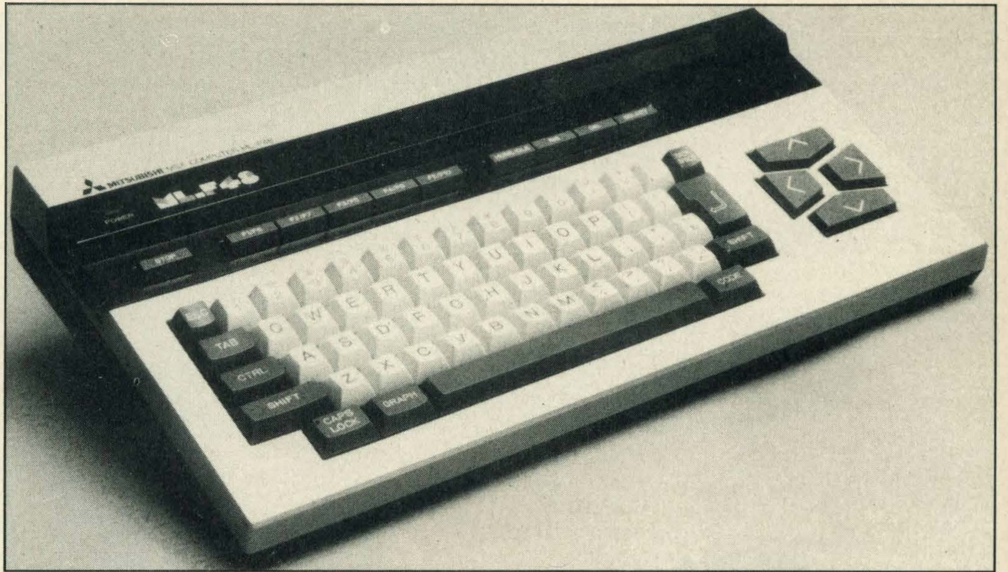
A 32K Mitsubishi ML-F48 has the same memory for BASIC programs as a 64K system
