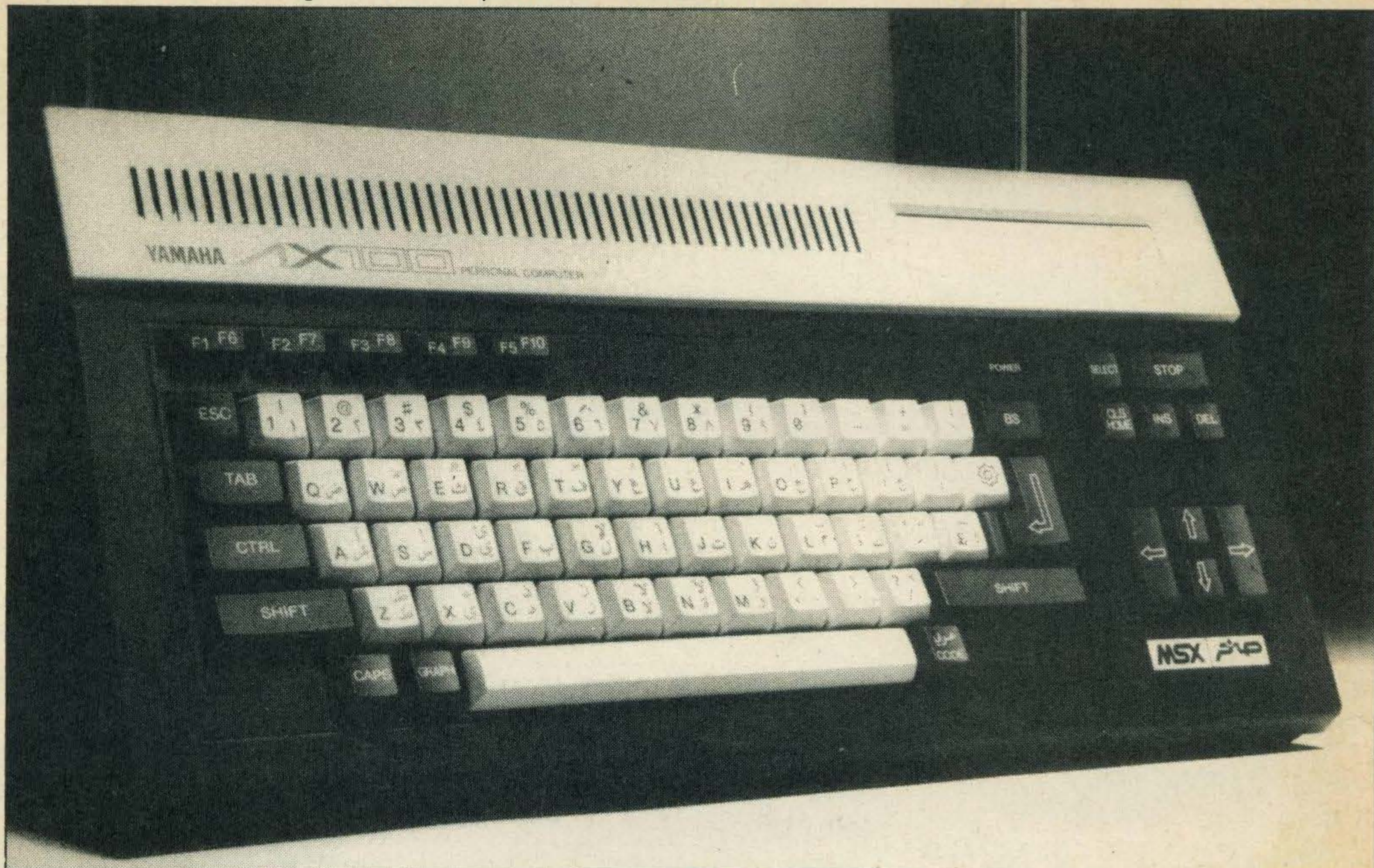
The Yamaha AX-100 is the first completely bi-lingual MSX computer to go on sale.
