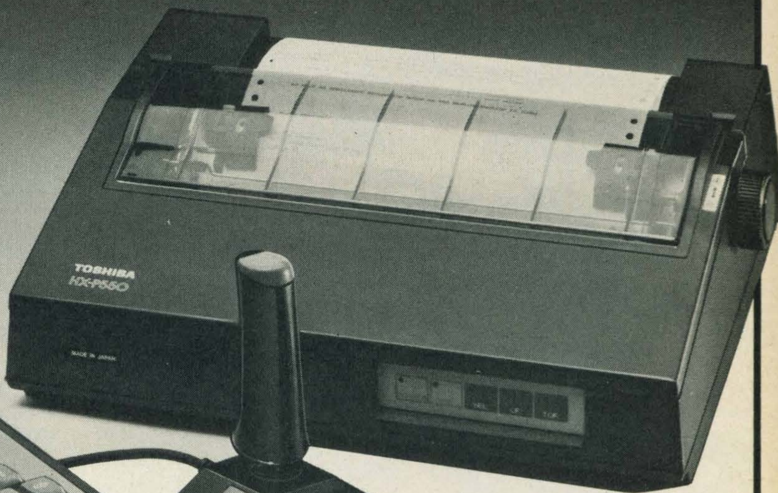
HX-P550 HIGH SPEED DOT MATRIX PRINTER Printing at 105 characters per second, for fast copies of all information, including graphics symbols. Ideal for word processing and programme listing. £349.00
