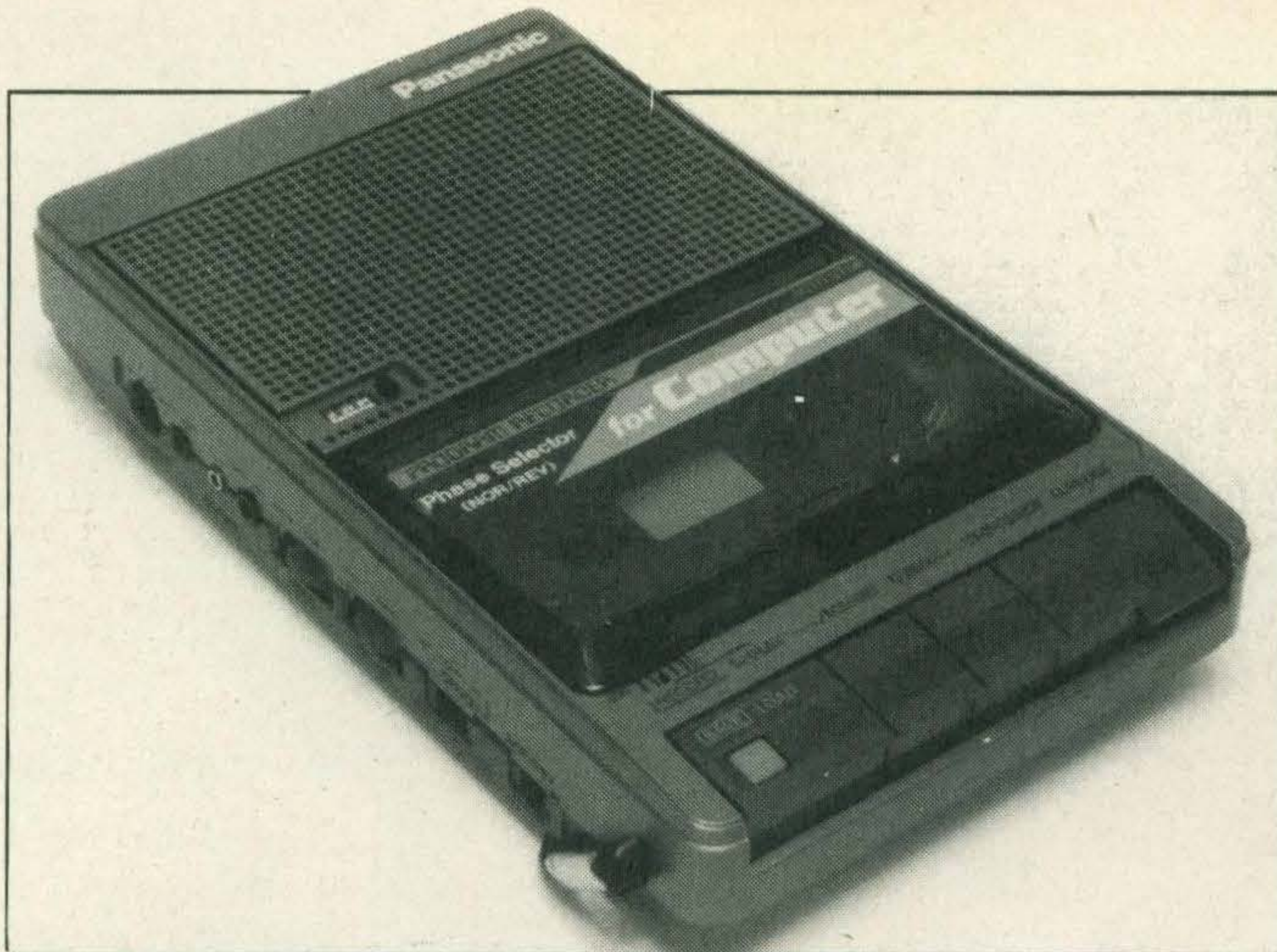
RQ8100 data recorder is battery powered, compact and costs £44.50
