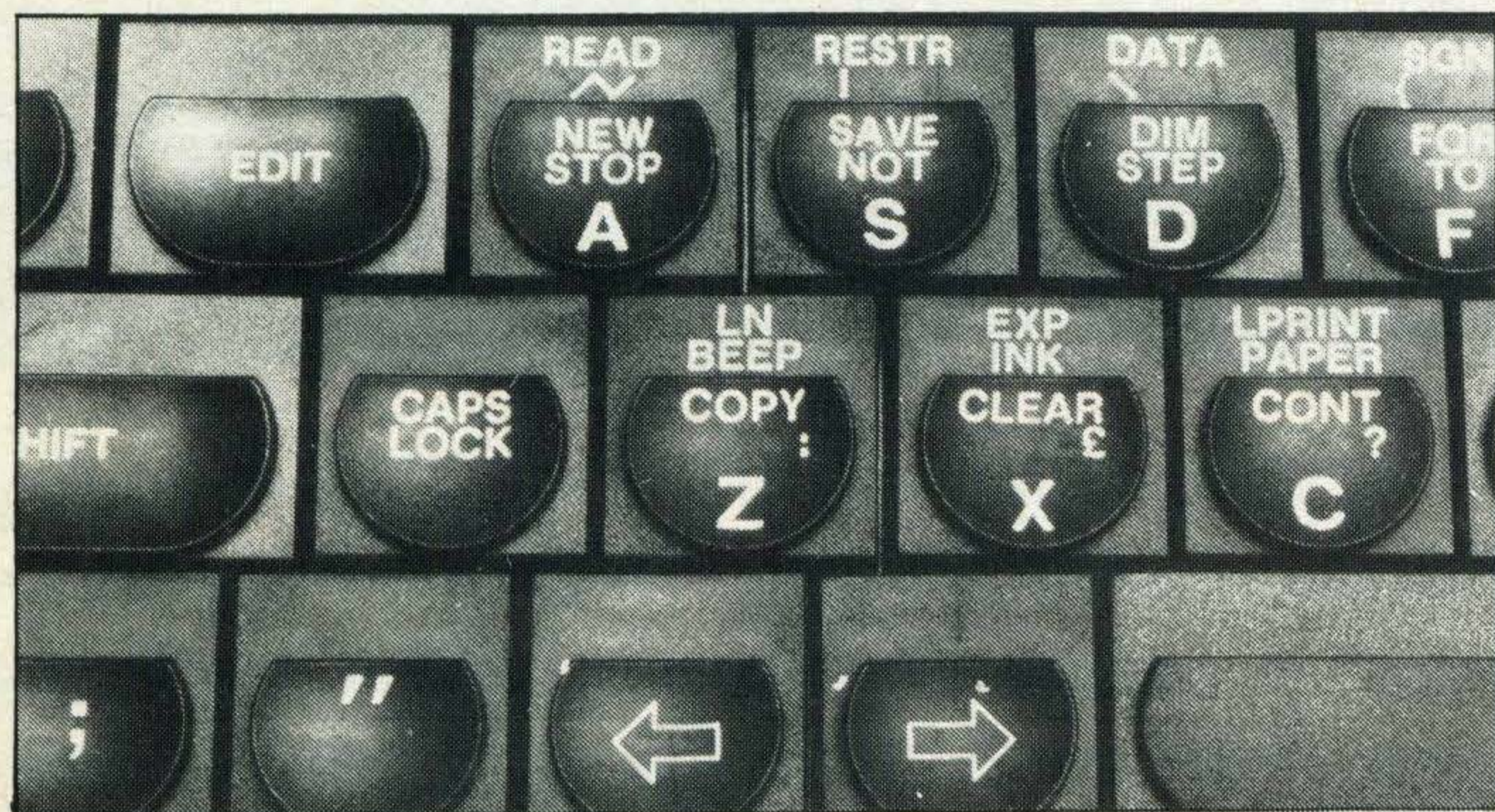
Spectrum has single key entry of BASIC keywords. It takes getting used to
