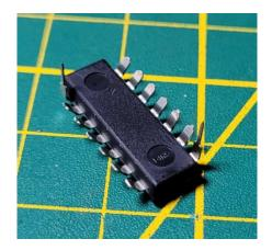
Then solder this chip on top of the U45 chip on the motherboard. Make sure that you correctly position the new chip before soldering. Put some solder onto the pins 1 to 6 - this will be necessary to solder wires to them later.
