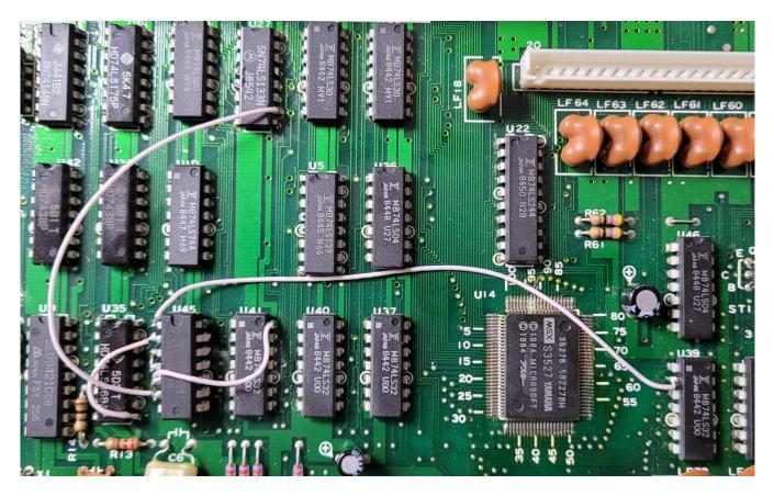
On the back side of the board it's necessary to solder only one wire from pin 25 of the cartridge slot to pin 2 of the U39 chip. Below is the picture of the completed wiring on the bottom side of the motherboard:
