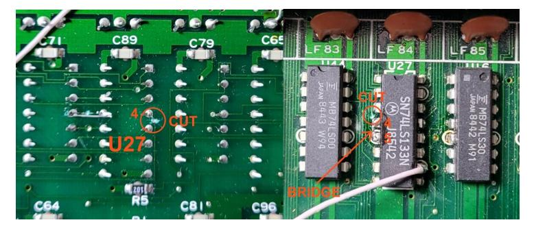
And finally, a few wires need to be soldered on the top and bottom sides of the motherboard to complete the fix. The following connections need to be made:
